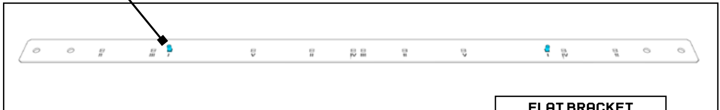
TAPE FROM BOTTOM TO HOLD BOLT IN PLACE
