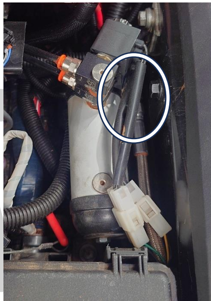
Figure 42. Compressor to manifold hose connection
