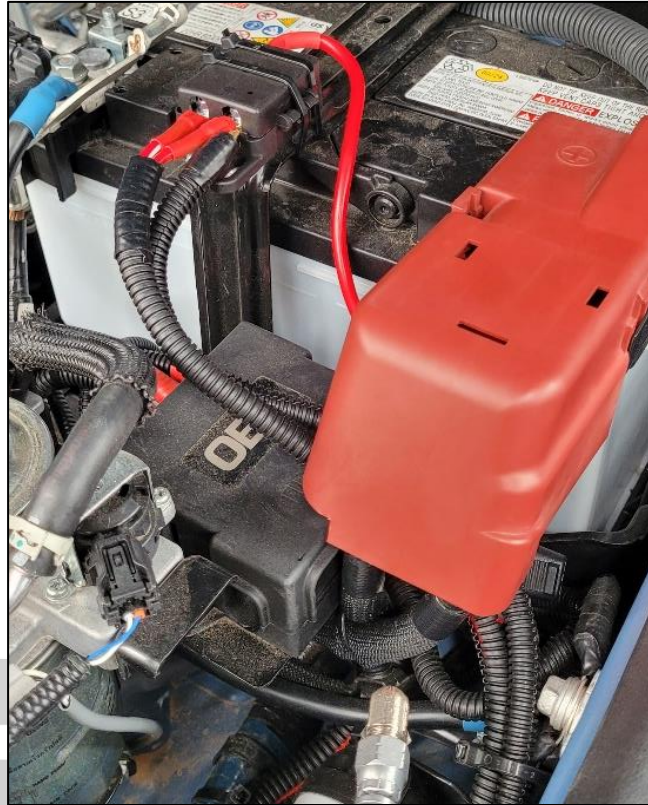
Figure 43. Recommended mounting location for compressor fuses
