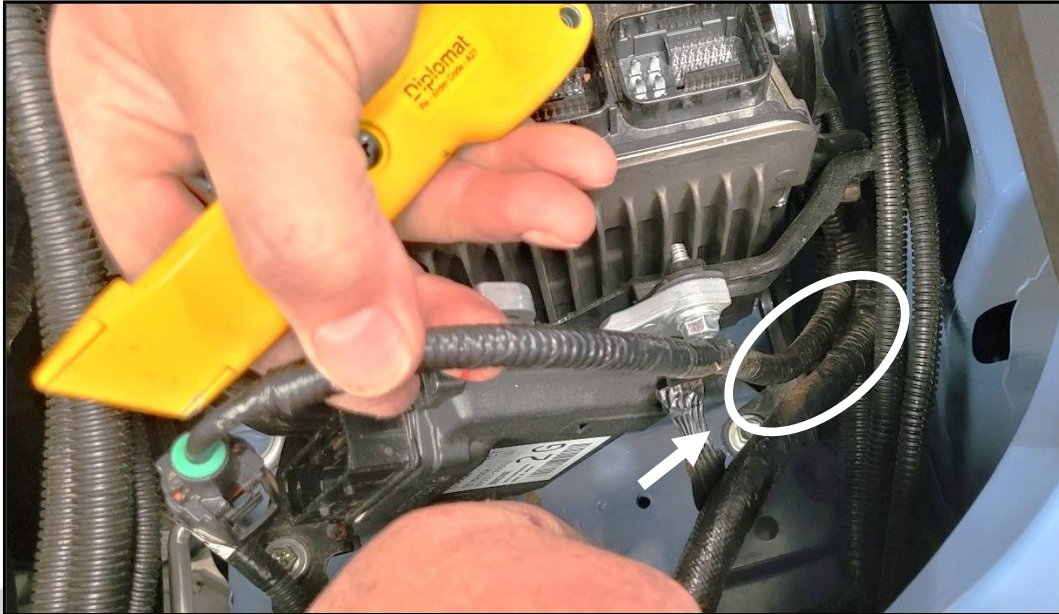
Figure 7. Cut tape to allow harness separation
