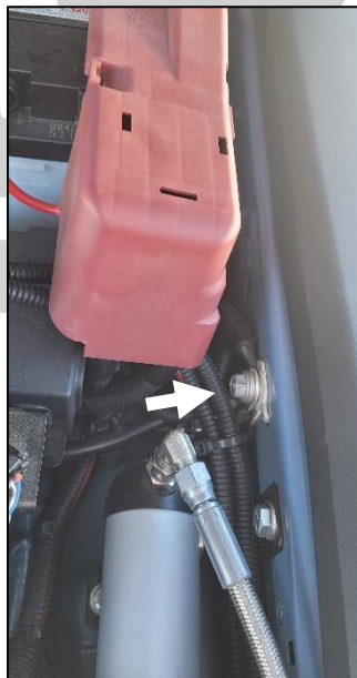
Figure 44. Preferred body grounding point
