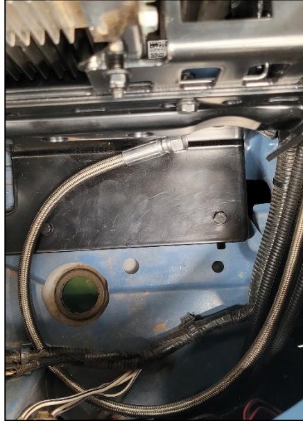
Figure 41. Compressor end of the braided hose
