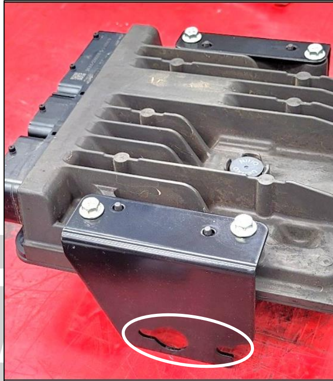
Figure 11. Correct orientation of ECU brackets
